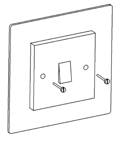
5. Push the light switch back against the wall ensuring the screw holes are lined up, then screw in both screws.
